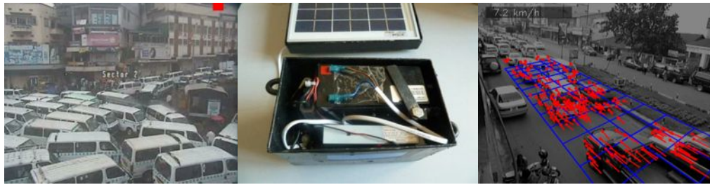
Figure 5: (left) traffic congestion in Kampala; (centre) low cost, solar, cameraphone-based traffic monitoring unit; (right) video analysis of traffic flow from solar unit.
